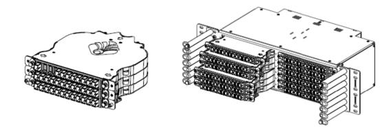
Splitters are housed inside some type of enclosure. Clearfield uses the Clearview Cassette. A cassette and each splitter leg are loaded into the rear of an adapter. This allows jumpers to be plugged into the front of the cassette.
