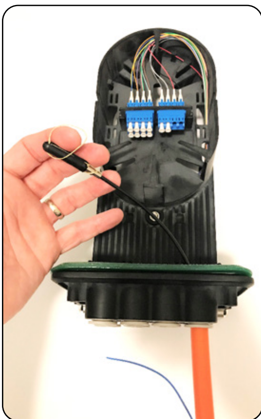
Microduct with Pushable Fiber
