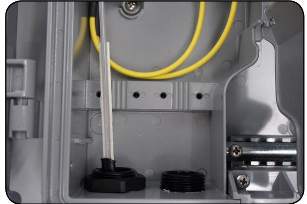
3. Place the strength member clamp(s) on top of the strength members, and tighten until fully secured.
