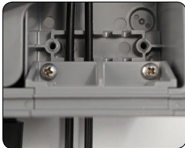
7. To secure the cables, install the v-clamp provided with the box. Using the two screws, tighten the v-clamp into the base of the box, allowing the edges of the clamp to grab the jacket of the cables.
