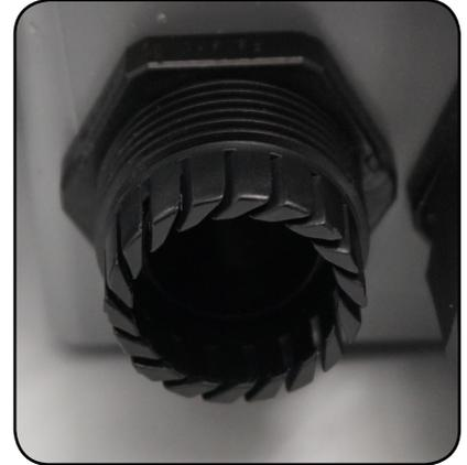
2. Remove the filler plugs from the holes in the grommet as needed. Slice the wall of the grommet in the locations where flat drop will be installed.
