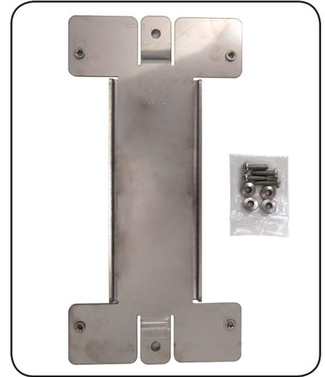
When installing the mounting bracket onto a metal pole, utilize two band clamps, supplied by the customer. Each clamp will slip through the two adjacent slots in the underside of the mounting bracket. Once both are through the mounting bracket, secure the bracket to the pole using the band clamps.
