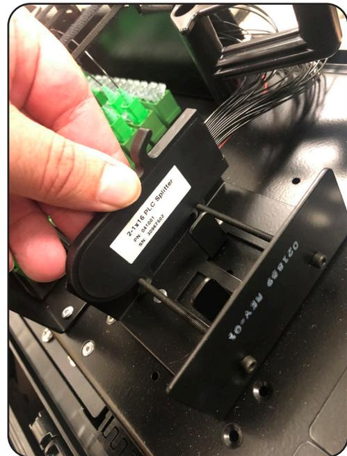
2. To secure the splitter body into place in the 288 Port Aerial FDH, swing the locking arm over the top of the splitter cage and lock it into place with the latch.
