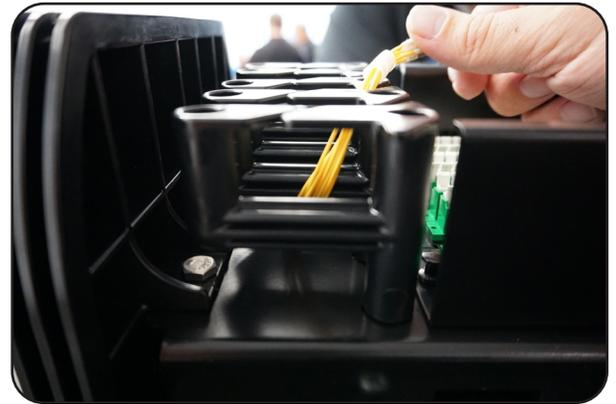
6. Once a proper amount of the slack has been taken up, transition up to above the crossbar of the rods, reversing direction.
