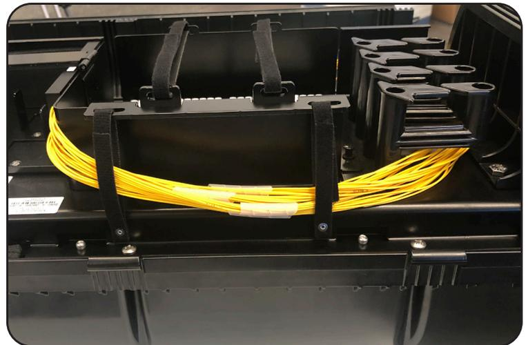
4. Bring the staging plate down and around to the staging area. Allow the splitter legs to route underneath the fiber management. Using the push/pull plungers on the staging plate, install it into the blank staging area down below the distribution ports. Press on the plungers once they are through the holes on either side of the staging area to lock it in place.
