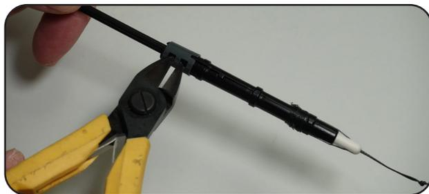
2. Cut the pull string wrapped around the front end of the bullet to separate the halves of the bullet from the SFF.
