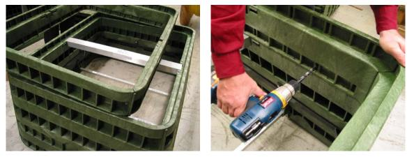
7.3 Insert bolts with flat washer through the mounting holes. Add remaining flat washer, split ring lock washer, and nut, and tighten until secure.
