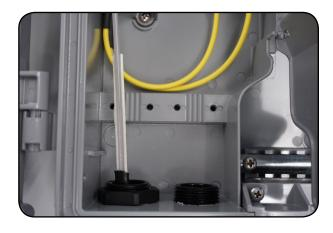
**3.** Place the strength member clamp(s) on top of the strength members, and tighten until fully secured.
