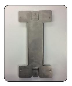
When installing the mounting bracket onto a metal pole, utilize two band clamps, supplied by the customer. Each clamp will slip through the two adjacent slots in the underside of the mounting bracket. Once both are through the mounting bracket, secure the bracket to the pole using the band clamps.
