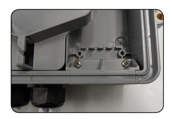
**2.** Remove the cable retention grommet.
