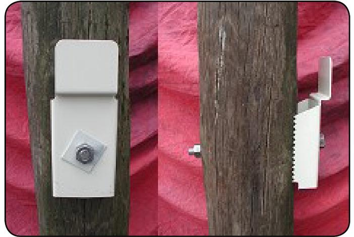
**Note:** Clearfield does not recommend using lag bolts to mount cabinet to pole. Clearfield recommends using hardware with a minimum of 5/8" diameter. Care should be taken to avoid over-tightening and deforming the hoist plate. Lock tight (red) should be used on nuts to prevent loosening of nuts. Make sure the thread rod/nut does not exceed the top bend in bracket or it will interfere with cabinet.
