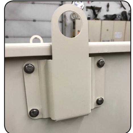
2. Install one of the mounting brackets with teeth to the bottom of the cabinet on the side of the cabinet that will face the wall, using the pems on the cabinet riser and the hardware provided.
