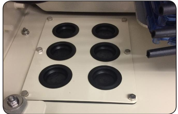
2. If the entrance plate already has a cable installed, you will need to loosen the sealcon's dome nut. This will allow the plate to slide along the pre-installed cable.
