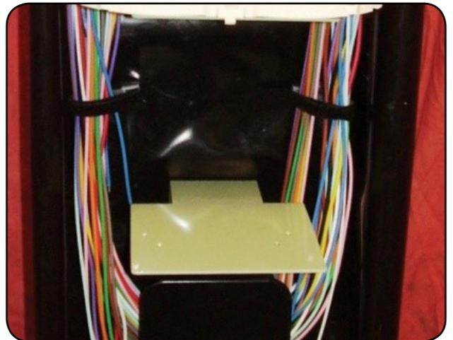
5. The first sacrificial splice tray is pre-installed with two 4-40 x 1/4" screws (part number 001523).
