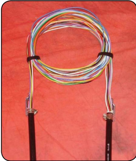
**Ring cut/Mid-span opening**
