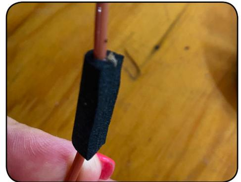
3. If applicable, open the buffer tube. Place the rubber strain relief boot into the splice tray, then tie the buffer/fanout tube into the tray with a small cable tie or wax string.
