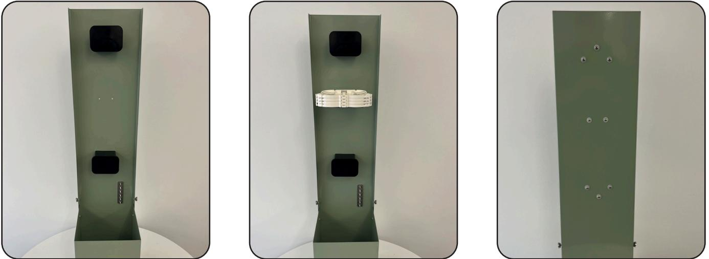
The FiberFirst Metallic Pedestal is capable of holding up to 144 splices by adding up to twelve 12 fiber trays to the included bracket. With the addition of a second splice tray bracket, the FiberFirst Metallic Pedestal can accommodate up to 288 splices.
