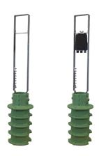
The FiberFirst 6-Inch Pedestal consists of a two-part base and removable cover measuring 5.9" in diameter and 30" in height and is designed and tested to withstand harsh environmental conditions, as well as UV, chemical and impact resistance. The pedestal includes a built-in, multi-use metal frame for mounting various products inside the pedestal. An industry standard telco security screw (216) is used to attach and lock the cover to the base.
