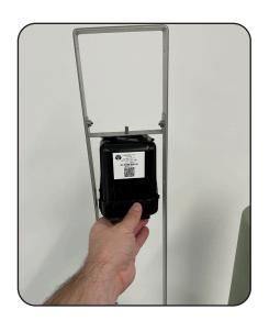
**2.** Using the wing nut, secure the SeeChange Terminal into the pedestal.
