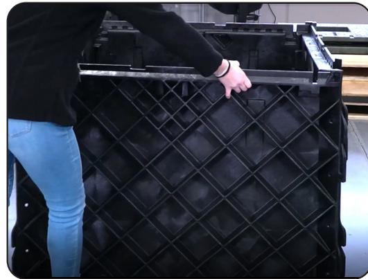
3. Secure the walls together using the 8 wall clips (2 per side). Following the direction of the arrows on the outside of the clips, slide the channel of the clips down over the flanges on the corners of the walls.
