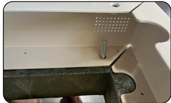
3. Secure the riser/ped to the lid with the provided washers and nuts on the J-hook bolts.
