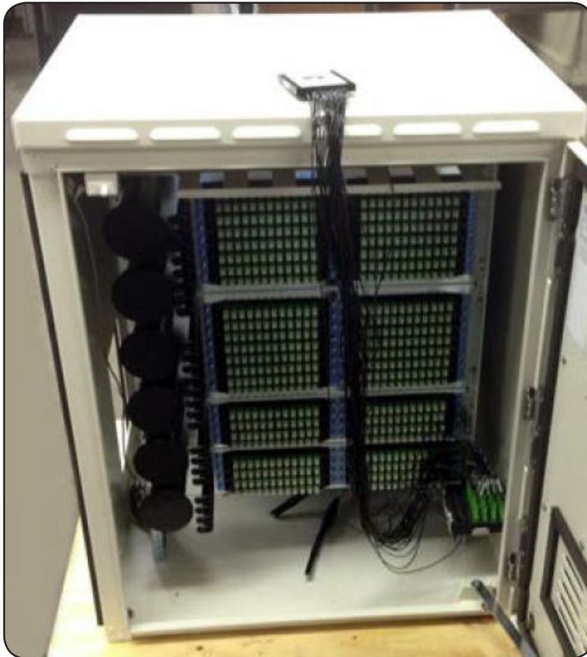
**Step 8:** Route each PON-side fiber from the staging plate to the appropriate position on the fiber assembly and terminate the fiber. Begin with the lower right assembly, and then proceed to the lower left assembly, populating each assembly in sequence with the top left assembly populated last.
