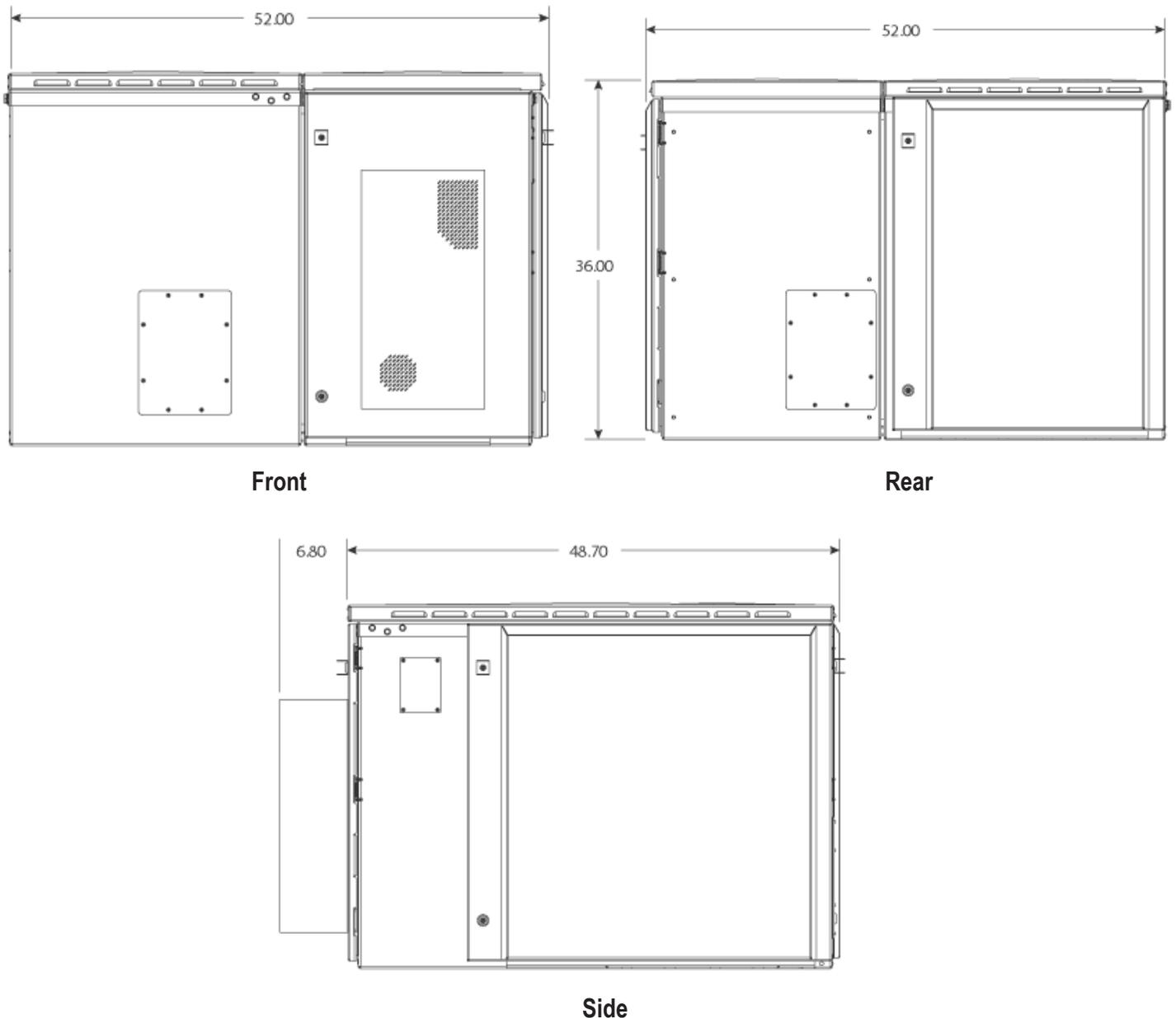
**Note:** For clearance and space requirements when mounting the EXM on the rear or side of the base FAC 900 cabinet, refer to Space Requirements.
