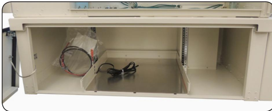
Clearfield provides an optional AC line operated 150W battery heater mat which turns on at 40°F to increase battery capacity in cold environments. Battery mats are available in 120VAC and 240VAC versions.
