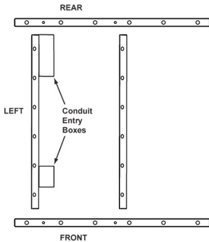
**Step 3:** Attach the short and long brackets together using eight supplied screws and nuts, as shown.
