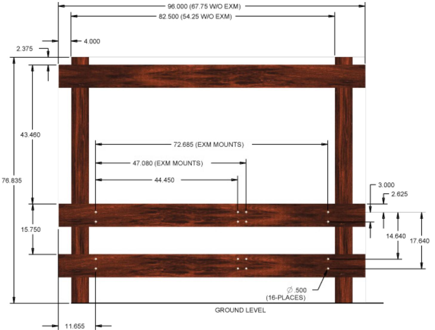
**Wall/H-Frame Mount Dimensions: High Profile Configurations**
