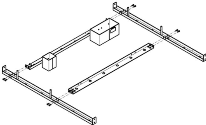
**Step 4:** Tighten all screws to complete the template assembly.
