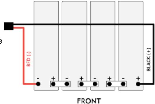
**ALERT!** Use a volt meter to verify correct wiring polarities.
