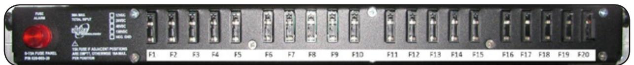
Install a 2A GMT fuse in position 20 and verify that the heat exchanger fans start running (if internal temperature is high enough).
