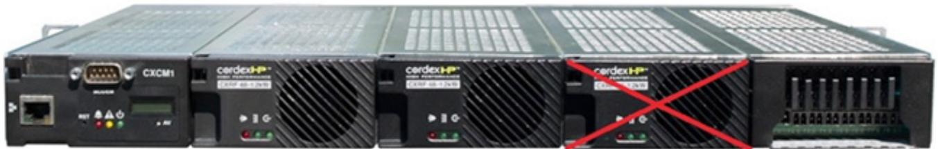
**Note:** The far right slot does not support a rectifier module.
