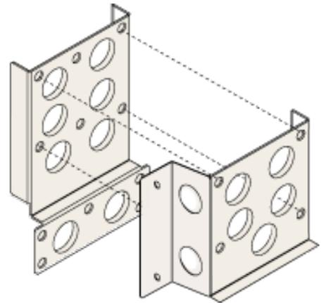
**Step 4:** Install the cabinet on the mounting fixture.
