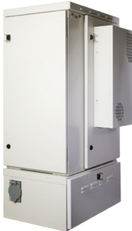
The FAC 400 cabinet has a single compartment that houses electronics equipment together with fiber and copper plant terminations, enabling deployment of multiple applications from one node. The electronics area is equipped with a vertically-oriented 19-inch equipment rack that provides 4 RU of mounting space.
