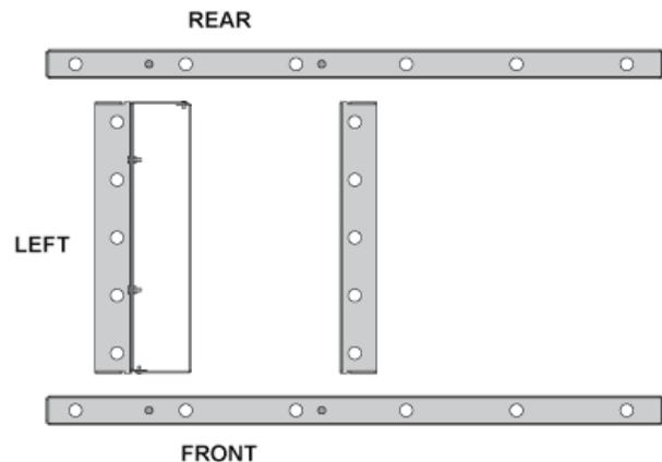
**Step 4:** Attach the short and long brackets together using seven supplied screws and nuts, as shown.
