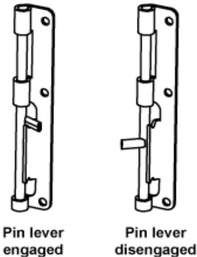
**Step 5:** Release the hinge pins from the hinge pin channels as follows:
