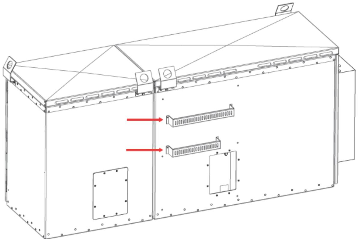
3. Route the cables and splices from the main equipment compartment through the rear access hole to the cable dressing bars.
