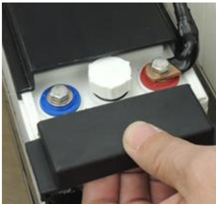
4. At the unattached end of the jumper, wrap the lug with electrical tape.
