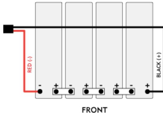
**ALERT!** Use a volt meter to verify correct wiring polarities.
