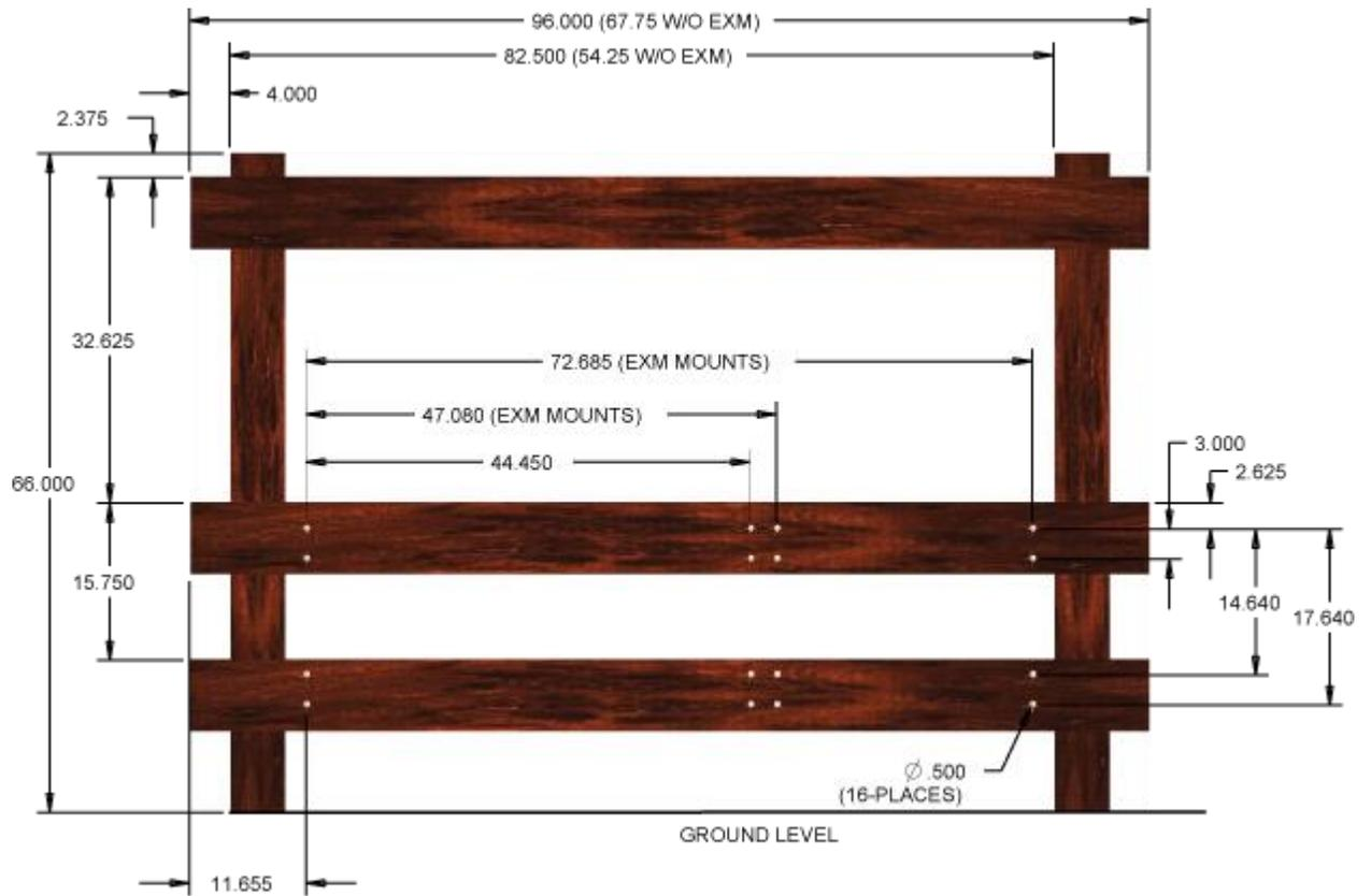
**Wall/H-Frame Mount Dimensions: Low Profile Configurations
