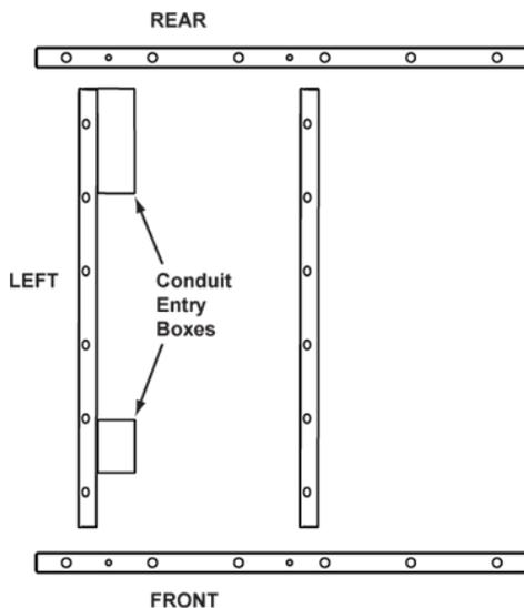
3. Attach the short and long brackets together using eight supplied screws and nuts, as shown.
