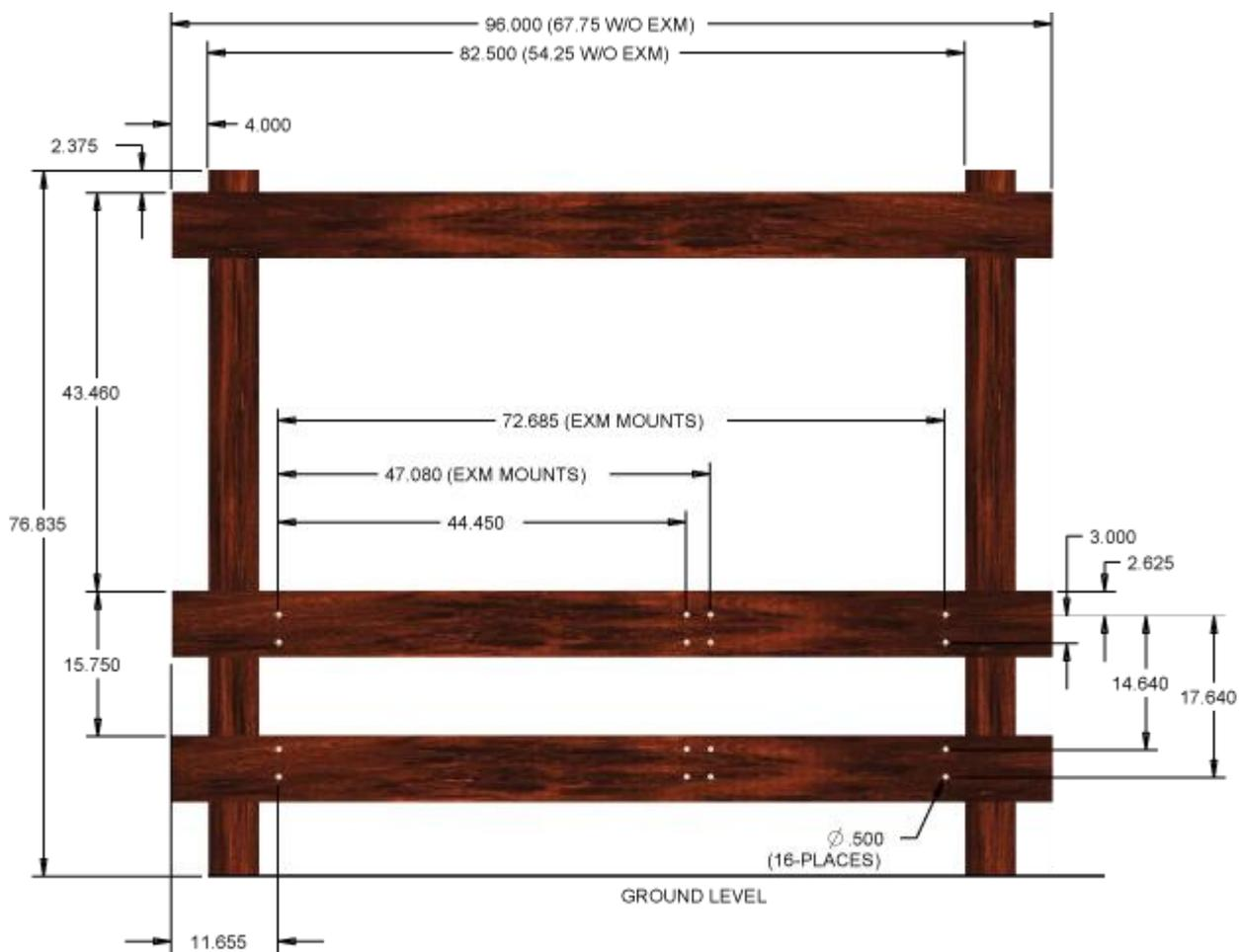
**Wall/H-Frame Mount Dimensions: High Profile Configurations
