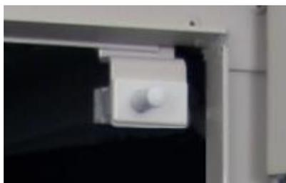
**Note:** Do not rotate the switch plunger. Rotating the plunger may damage the switch.
