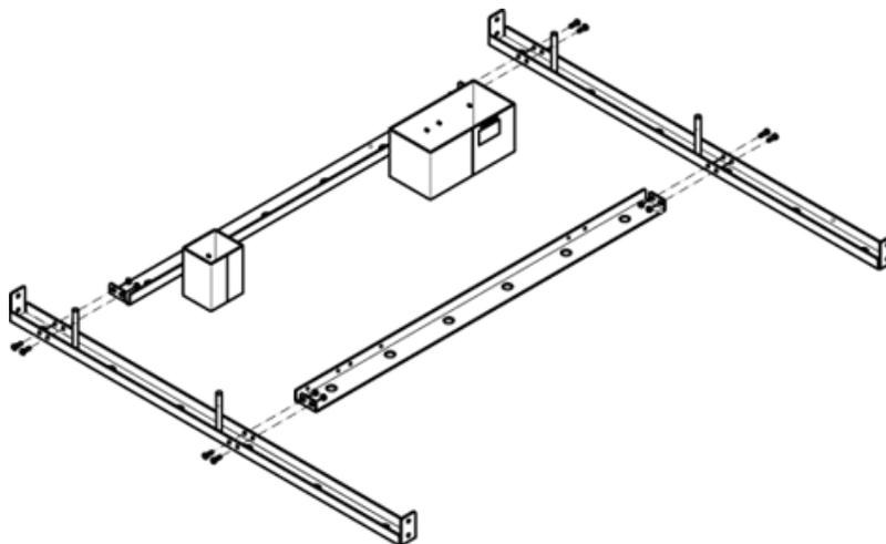
4. Tighten all screws to complete the template assembly.
