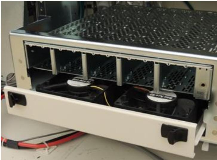
4. Slide the fan tray completely into the slot. Push firmly on the front panel to seat it.
