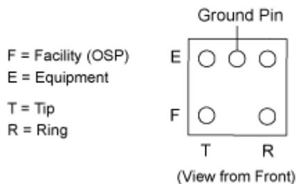
5. Using a volt meter, test between the Facility Tip and ground pins:
