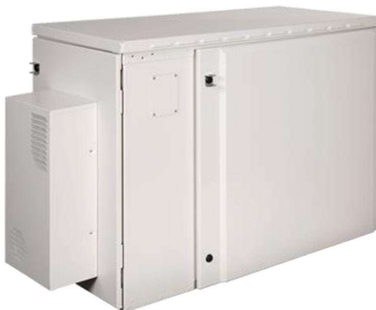
The base ODC-200 cabinet has a single compartment that houses electronics equipment together with high density fiber and copper plant terminations, enabling deployment of a broad suite of applications from a single node. The electronics area is equipped with a vertically-oriented 19-inch equipment rack that provides 8RU of mounting space, housing up to nine Calix E7-2 or B6-001 shelves and other 19-inch wide equipment.
