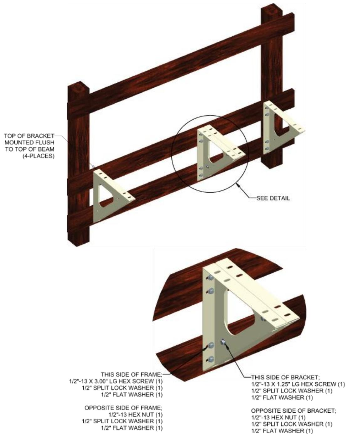
3. Attach the conduit feed through assembly to the wall/H-frame as follows:
