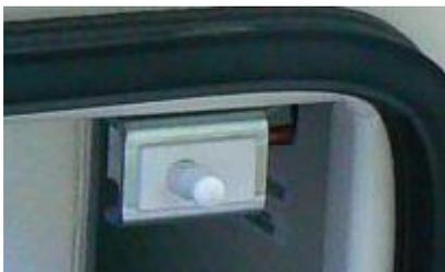
**Note:** Do not rotate the switch plunger. Rotating the plunger may damage the switch.
