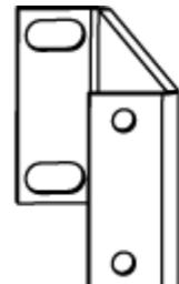
3. For equipment more than 1 RU high, install a second pair of projection brackets onto the rack, 1 to 4 RU below the first pair, using (2) self-tapping screws per bracket.
