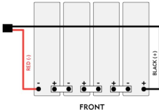
**ALERT!** Check all connections carefully to verify correct wiring polarities.
