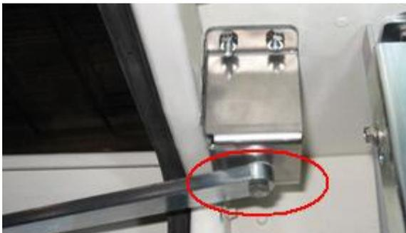
4. On the door hinges, disengage the hinge pin lever from its cradle:
