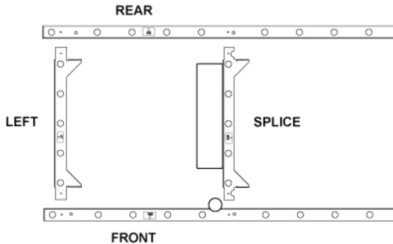
3. Align the Left bracket screw holes with the counterpart holes on the Front and Rear brackets.
