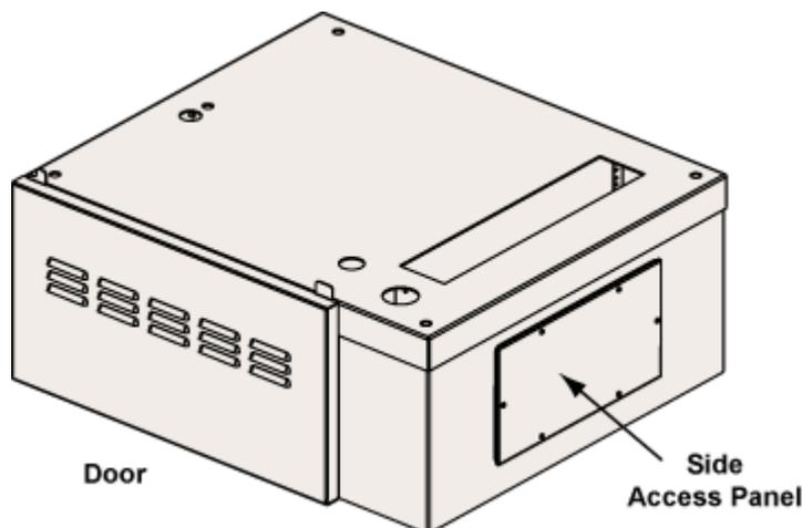
3. Remove the riser's side access panel. Use the Torx tool from the installation kit to remove the (6) Allen bolts.
