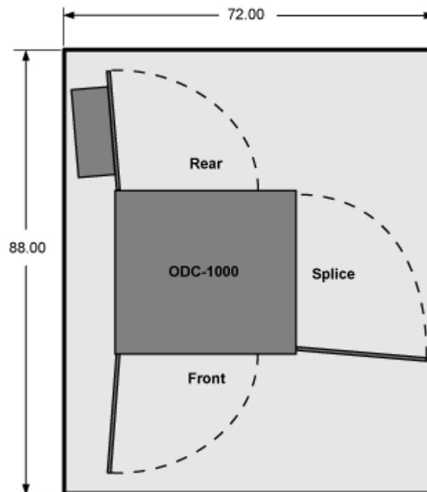
The minimum clearance area around the cabinet site must be free of permanent impediments to allow full swing of the cabinet doors. This area must be kept clear of obstructions at all times to provide adequate access for all installation and maintenance activities.
