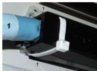
**Note:** To provide a securely-mated connection, be sure to align the head of the cable tie along the bottom edge of the RJ-21 connector as shown. Failure to install the cable tie correctly may result in an inadequate connection.
