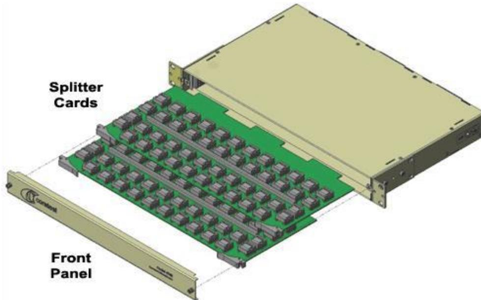
2. Pull the splitter card ejector tabs outward to the unlocked position.
