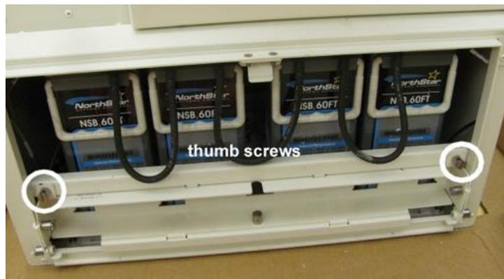
8. Replace the battery compartment door.
