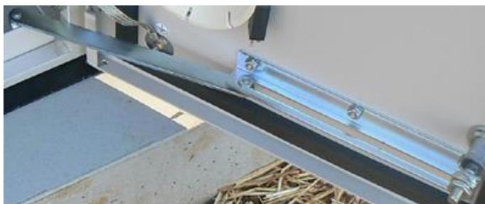
4. On the door hinges, disengage the hinge pin lever from its cradle:
