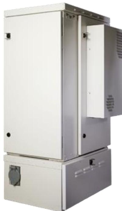
The ODC-100 cabinet has a single compartment that houses electronics equipment together with fiber and copper plant terminations, enabling deployment of multiple applications from one node. The electronics area is equipped with a vertically-oriented 19-inch equipment rack that provides 4 RU of mounting space. The ODC-100 houses up to three Calix E7-2 or B6-001 shelves, or up to two E5-100 service units.
