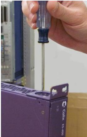
2. Attach the wall mounting bracket to the unit:
