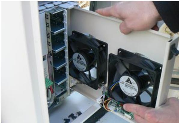
4. Slide the fan tray completely into the slot. Push firmly on the front panel to seat it.
