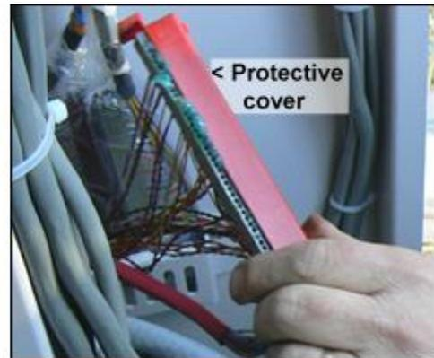
6. Install a protective cover over the mated MS<sup>2</sup> connectors.
