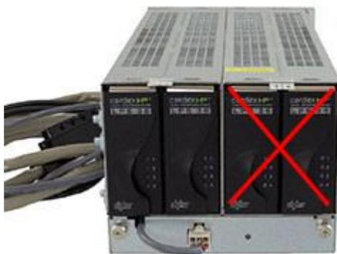
In this specific cabinet deployment model, the LPS36-4 up-converter shelf supports only up to two -48 to  $\pm 190$  VDC modules (eight line powering channels total) in slots 1 and 2. The number of converter modules required for operation varies by site based on several factors.
