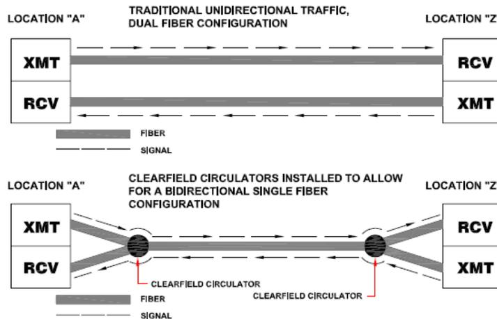
9. What is the difference between WBO & NBO? WBO stands for Wide Band Optics. Typically this is referred to standard WDM's using the much wider channel spacing having large channel passbands of +/-30nm, 40nm and 50nm. NBO stands for Narrow Band Optics. NBO refers to the CWDM 20nm channel spacing with a channel passband of +/-6.5nm.
