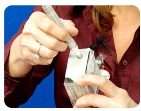
· Lightly touch short side of the MTP/MPO Connector Swab to the wetted area (3-5 secs) to absorb some cleaning solution (DO NOT over saturate the swab).
