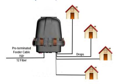
Example Above: Factory installed 150' 12 fiber flat drop toneable feeder with 4 SC/APC drops.
