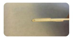
· Wipe connector areas to be cleaned, sliding pad from bottom of pad across and forward to tip of swab, from 1 side to the other, turn over and use long side to dry in same movement.
