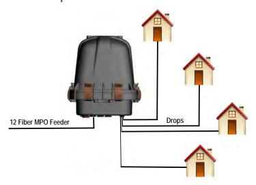
Example Above: 12 fiber MPO feeder with 4 SC/APC drops.
